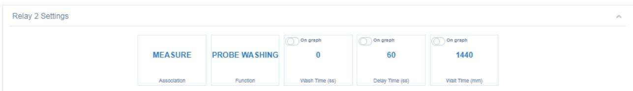
The bottom part of the 'Relay 2 Settings' window shows 'Association' (MEASURE) and 'Function' (PROBE WASHING). There are three 'On graph' radio buttons, all selected. The first is labeled '0' with 'Wash Time (ss)' below it. The second is labeled '60' with 'Delay Time (ss)' below it. The third is labeled '1440' with 'Wait Time (mm)' below it.
